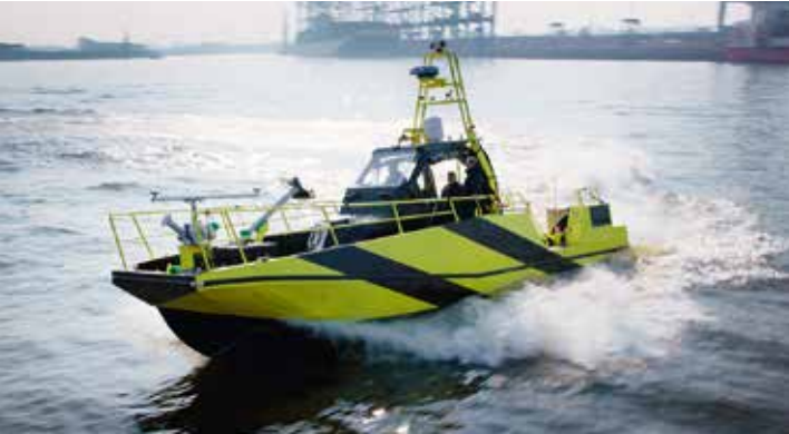
The AMC12 is a test bed for unmanned and autonomous surface ships that was developed in collaboration with partners.
