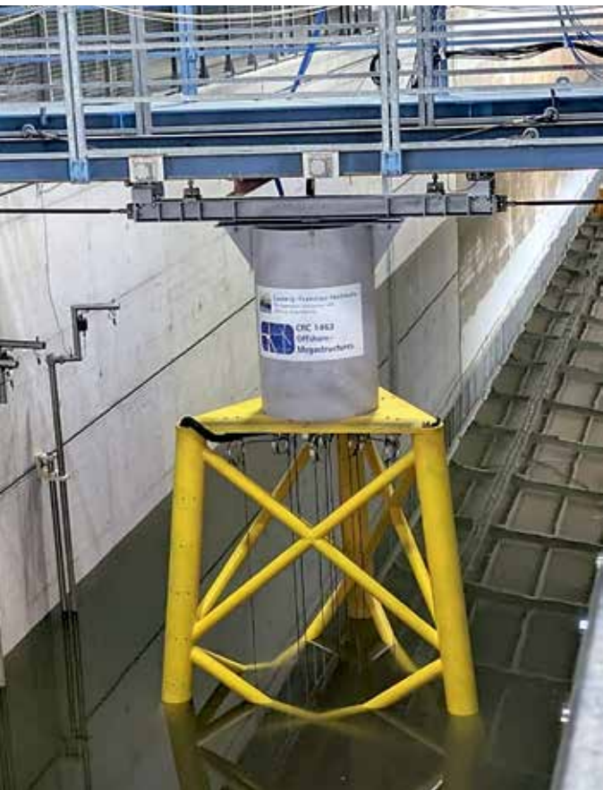
A 1:14 model of a jacket structure from the SFB. It depicts a foundation structure for an offshore wind turbine with a total height of over 300 metres.
