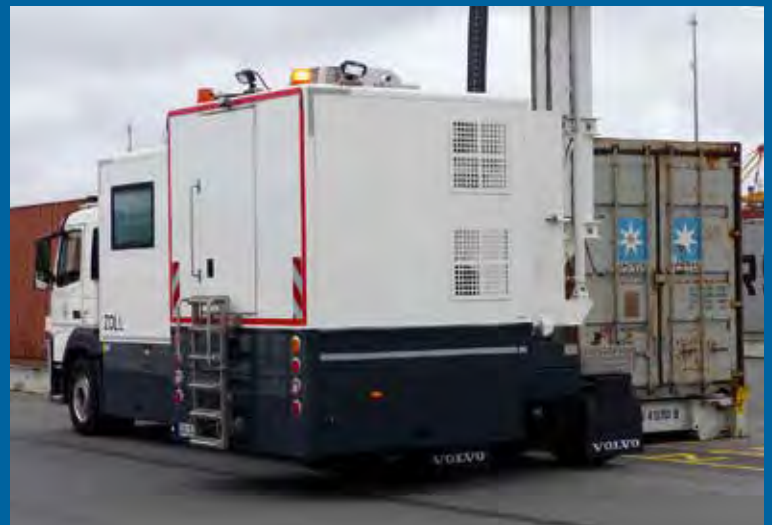
With a mobile X-ray system, customs can scan containers at terminals for different goods which the criminal believes are out of sight. This is not limited to drugs.
