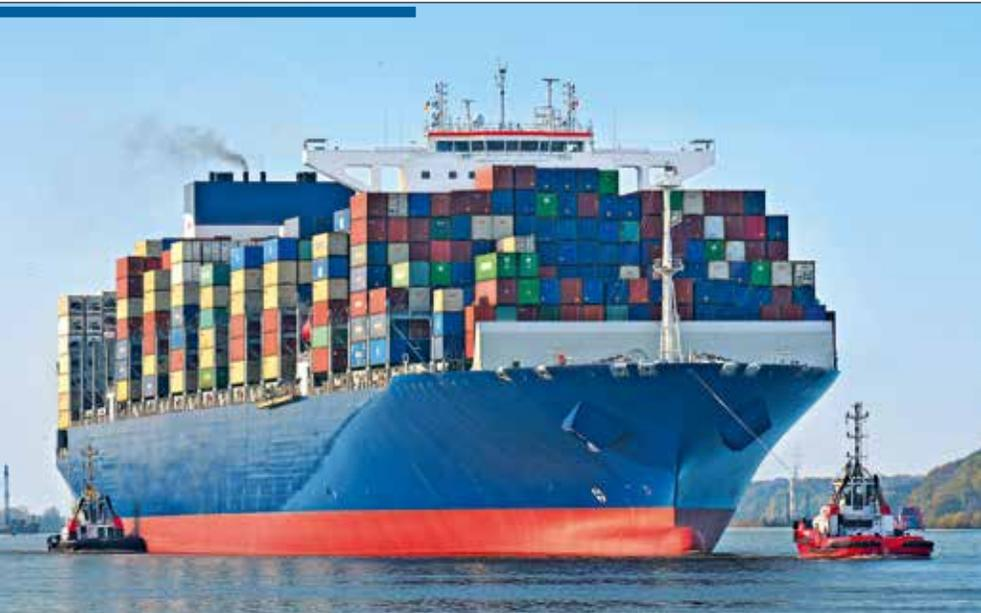
The number of tugs varies according to local conditions. For large Triple-E class container ships with 18,000 TEU, three tugs are usually required.
