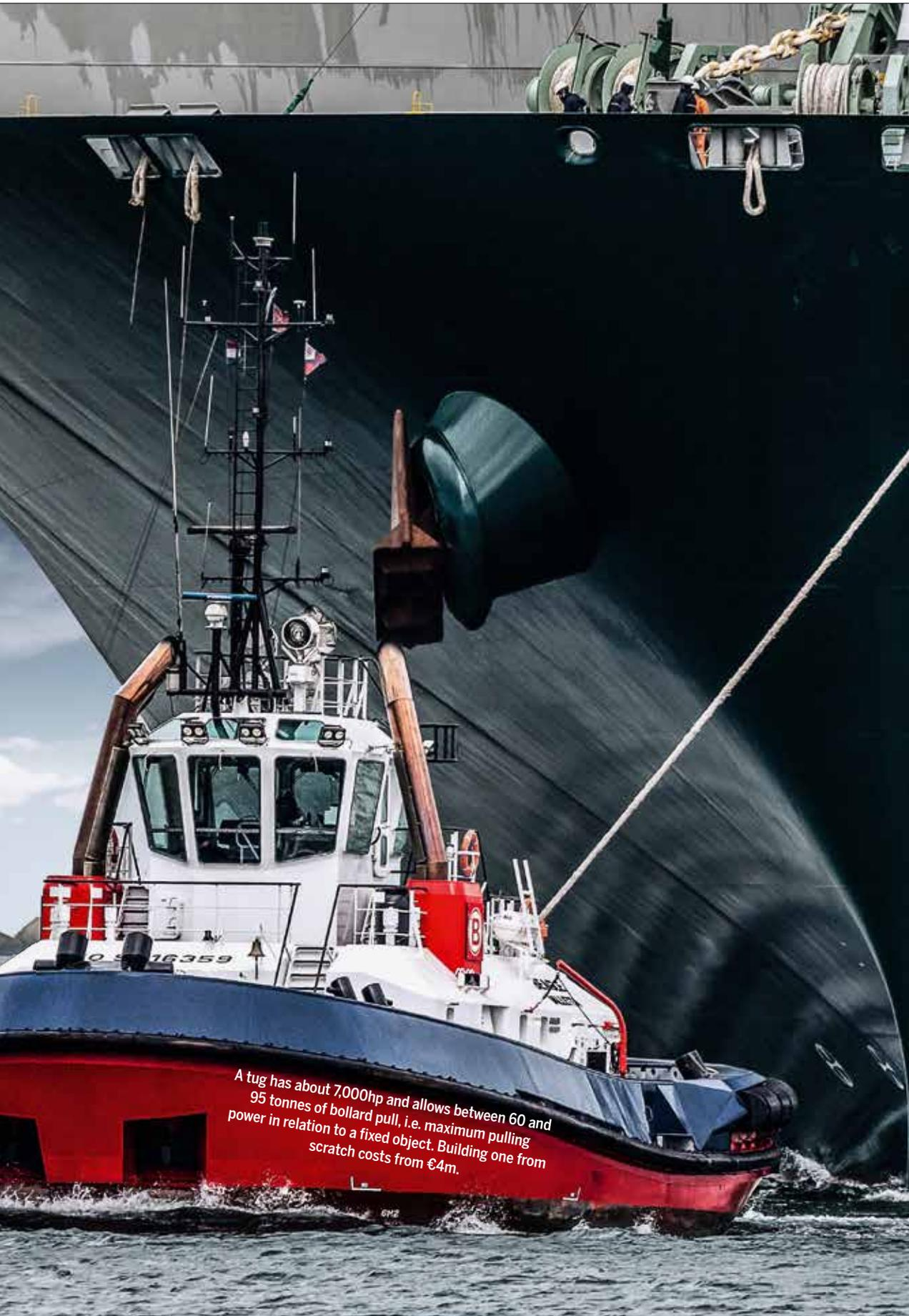
A tug has about 7,000hp and allows between 60 and 95 tonnes of bollard pull, i.e. maximum pulling power in relation to a fixed object. Building one from scratch costs from €4m.
