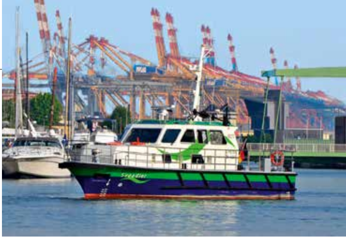
The Sea Eagle (left), launched in 2016, is part of the 'greenports' brand. It has a hybrid drive whose exhaust-optimised diesel engine enables fuel savings of 25 percent and significantly reduces emissions of nitrogen oxide and CO 2 . The bremenports fleet currently comprises eight electric and three hybrid vehicles.
