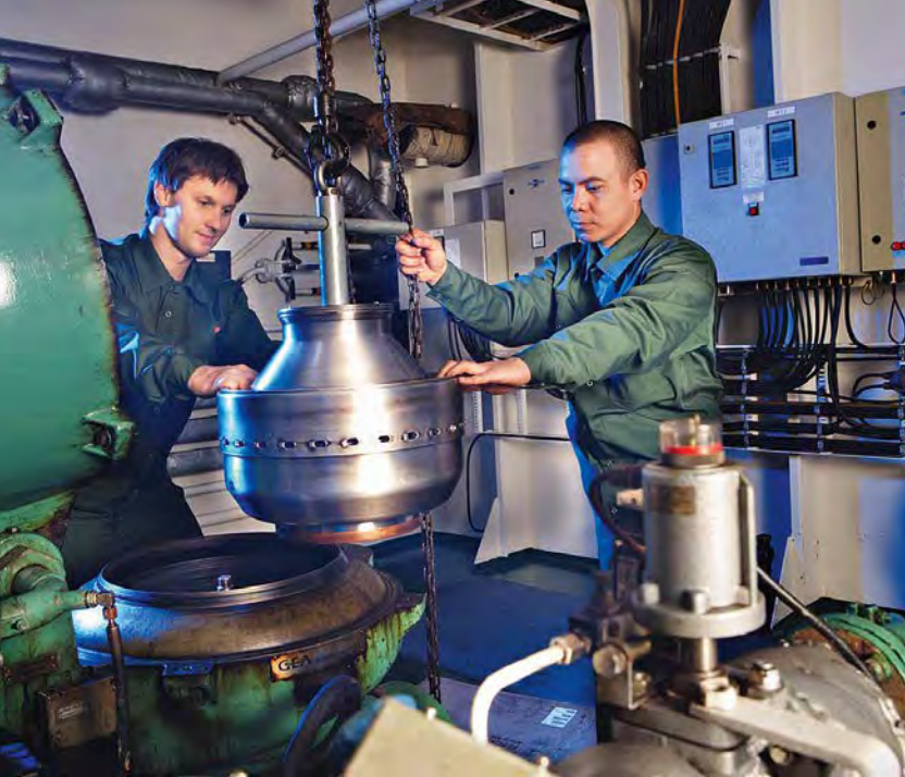
Cleaning and checking of the separator used to convert heavy oil into usable fuel.
