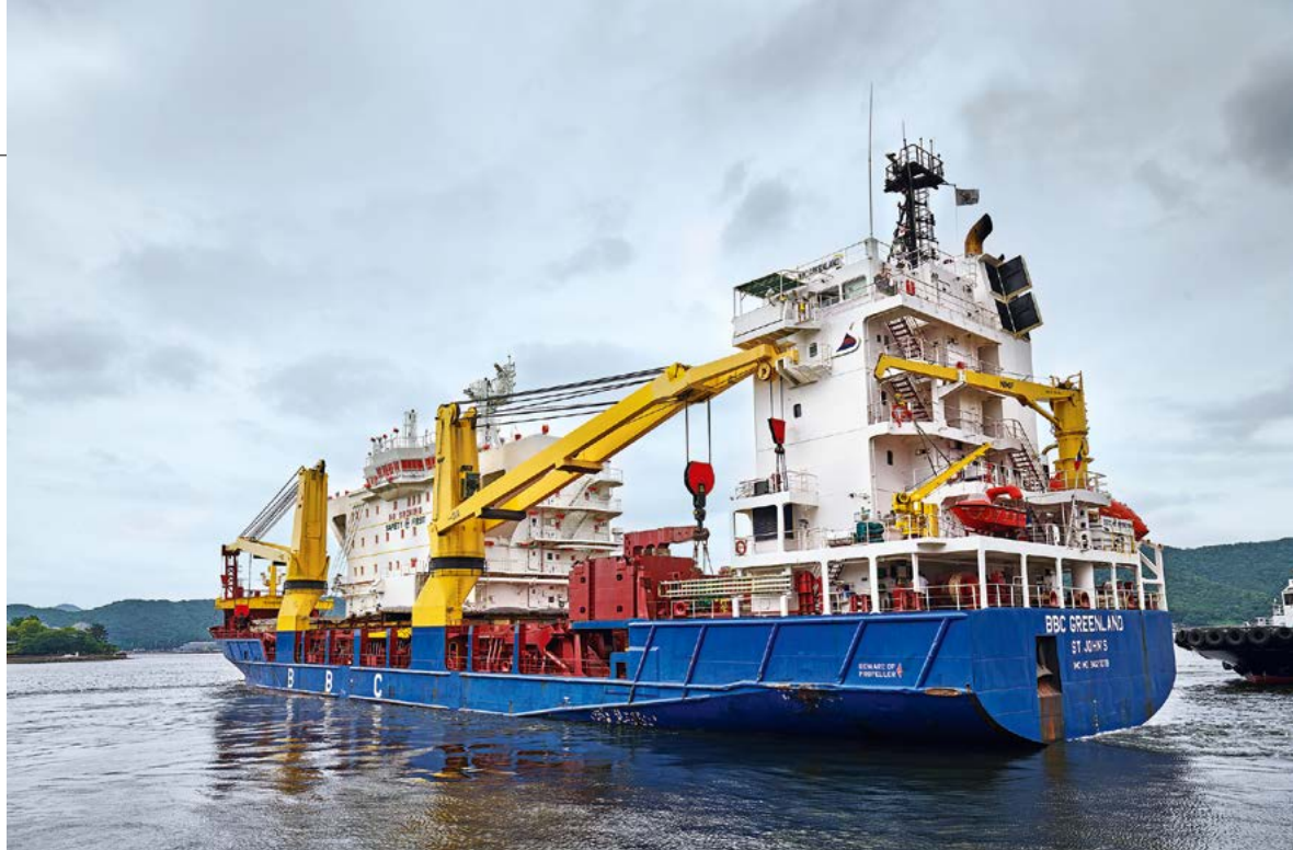
Transport of a deckhouse for FPSO units on the BBC Greenland. The cargo weighed about 830 tonnes.
