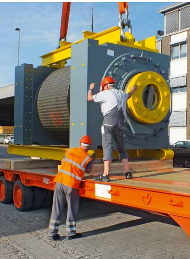
At the BLG AutoTerminal in Bremerhaven, the heavy rollers for the grinding plant in Mumbai were transferred from the train to a roll trailer and brought on board a ro-ro ship.
