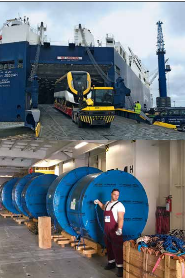
Static cargo with a high unit weight must be lashed on board elaborately with chains.
