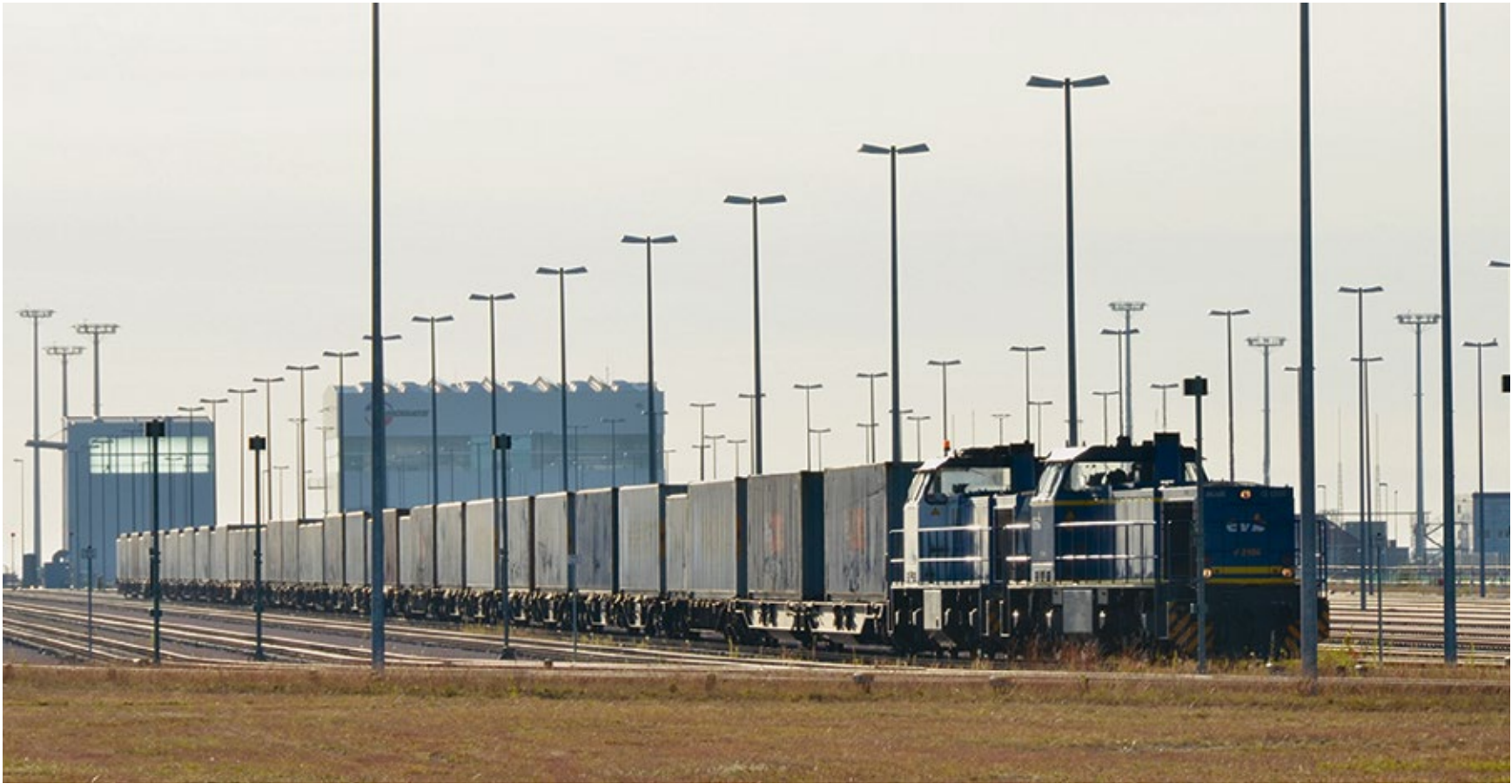
Expansive landscape of tracks: the 16-track formation sidings act as a buffer between the container port and the hinterland, with connections to key economic centres in Germany and the industrial regions of northern Europe.
