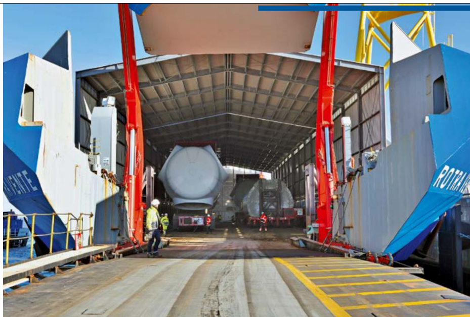
The transporter ship 'Rotra Vente' is 141 metres long and has capacity for several nacelles used in 8-megawatt turbines.
