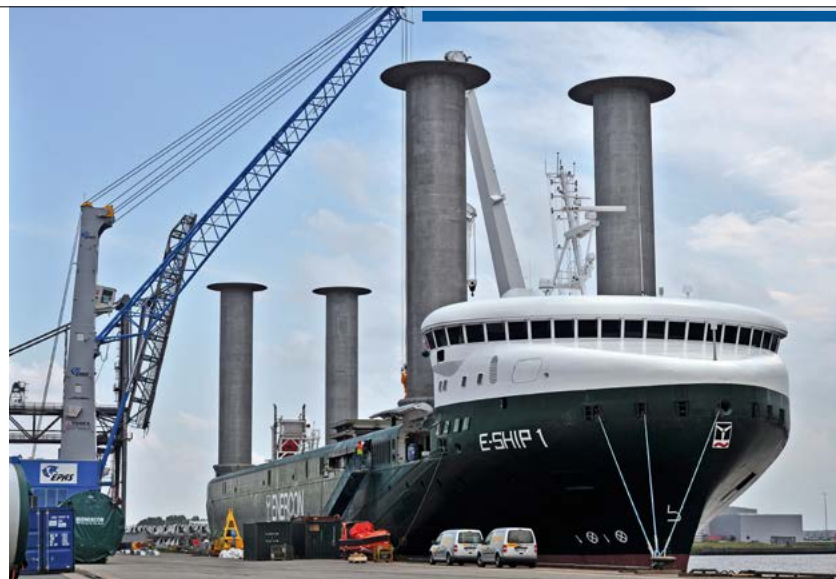
The project load ship “E-Ship 1” has Flettner rotors as well as a diesel engine. It is the world’s first commercial rotor sailing vessel.
