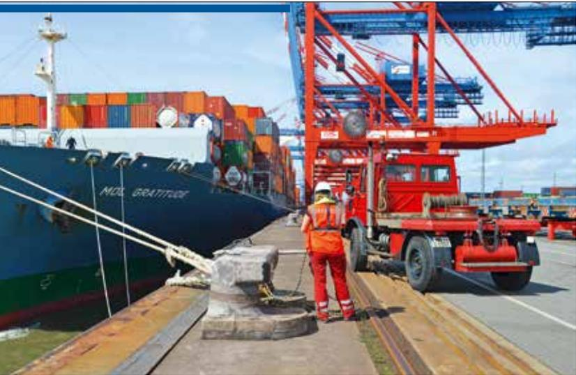
In addition to their physical strength, mooring lines also use specially equipped Unimogs with a 1.5-tonne winch.
